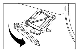
13. Lower the vehicle by turning the wheel wrench counterclockwise. Lower the jack completely.
